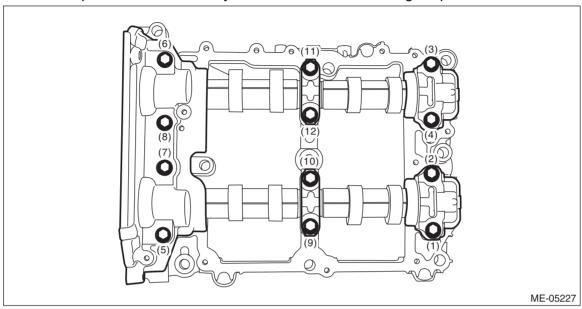
2) Remove the intake camshaft LH and the exhaust camshaft LH from cam carrier LH.
