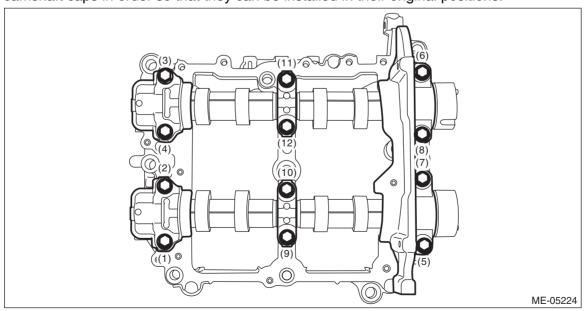
2) Remove the intake camshaft RH and the exhaust camshaft RH from cam carrier RH.
