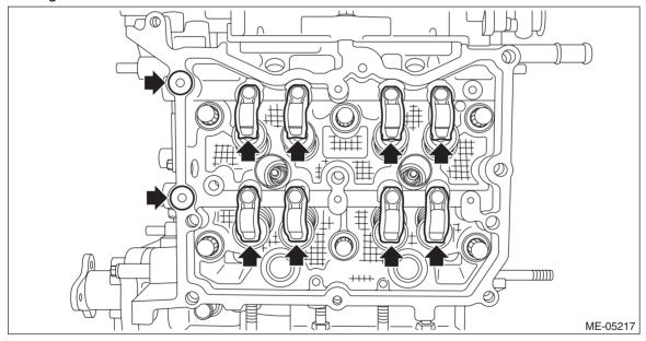
4) Apply liquid gasket to the mating surface of cam carrier LH as shown in the figure.
