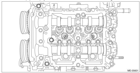
(5) Tighten the bolts (3 places) with a torque of 18  $N \cdot m$  (1.8 kgf-m, 13.3 ft-lb) in numerical order as shown in the figure.
