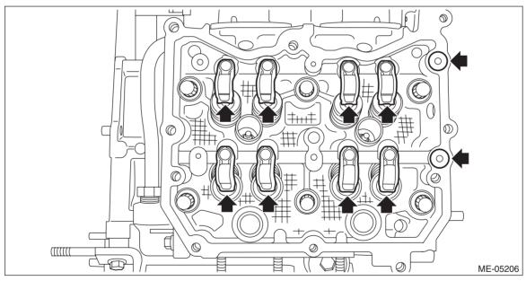
13) Remove the valve shim and the roller rocker arm pivot from cylinder head RH.
