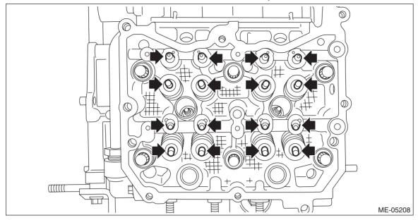
14) Remove the liquid gasket from cam carrier RH and cylinder head RH.
