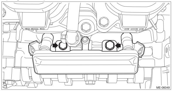
(2) Connect the quick connector to the fuel pipe RH.
