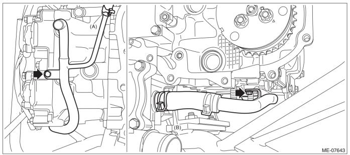
9) Remove the fuel pipe LH and the fuel injector LH.(1) Disconnect the connector from fuel injector LH.
