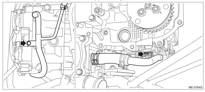
13) Secure the engine harness to the cam carrier LH with a clip.
