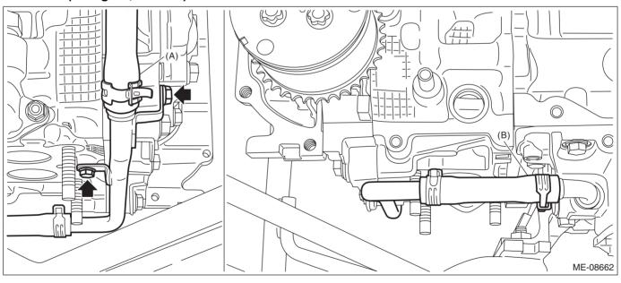
13) Secure the engine harness to the cam carrier RH with a clip.
