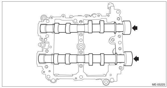
3) Remove the filter from cam carrier RH.
