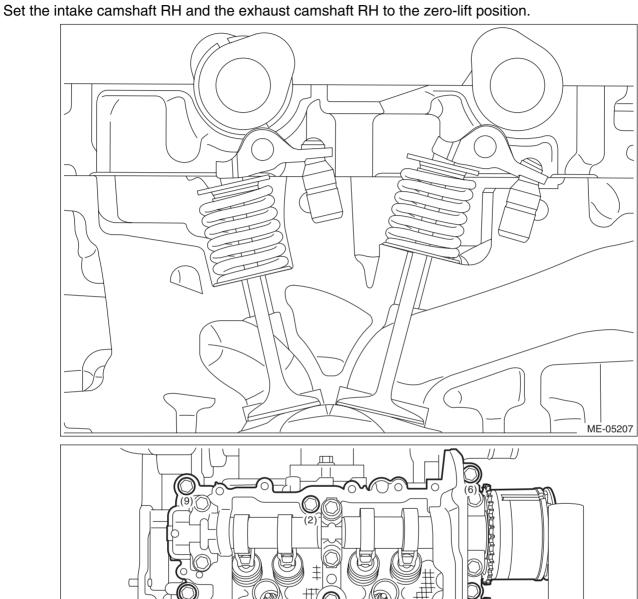
(2) Loosen the bolts (3 places) by 180° in numerical order as shown in the figure.
