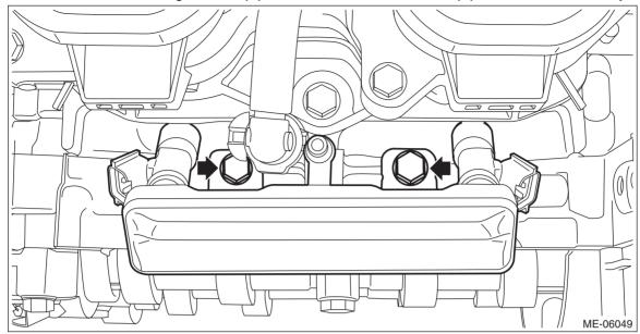
10) Insert the steel rods into ST, and set the engine so that the camshaft RH is facing up.
