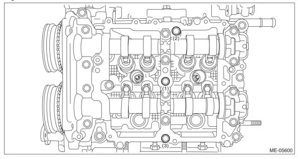
(4) Loosen the bolts (3 places) by 180° in numerical order as shown in the figure.
