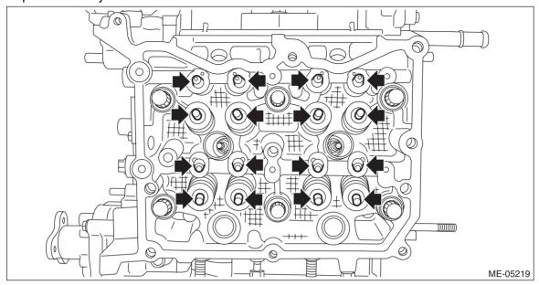
3) Apply engine oil to the O-ring and the roller rocker arm, and install the O-ring and the roller rocker arm to the cylinder head LH.
