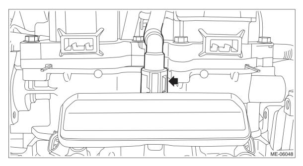
(3) Connect the connectors to the fuel injector RH.
