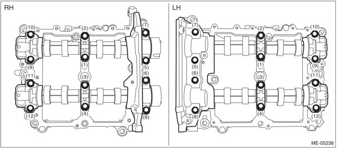
(6) Loosen the bolts (front camshaft cap, intake center camshaft cap, intake rear camshaft cap, exhaust center camshaft cap and exhaust rear camshaft cap) equally, a little at a time in numerical sequence as shown in the figure, and remove each camshaft cap.
