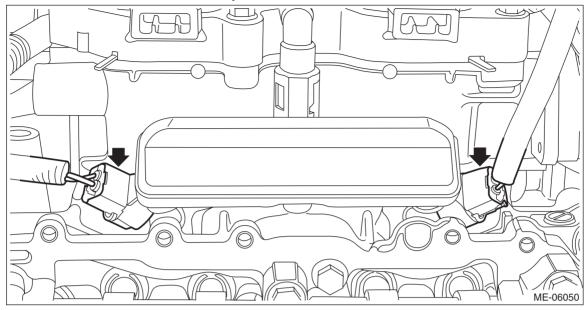
11) Connect the water pipe hose (B) to the oil pan upper, and install the water pipe assembly LH.
