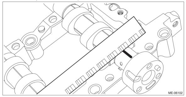
(8) Completely remove the plastigauge.
