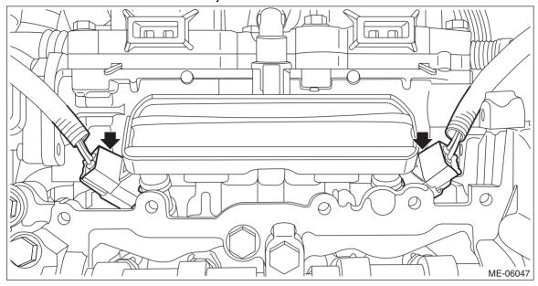
(2) Disconnect the quick connector from fuel pipe RH.
