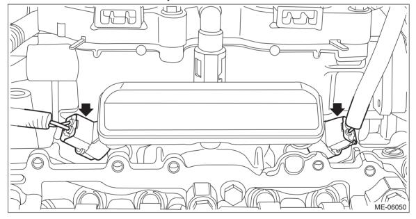
(2) Disconnect the quick connector from fuel pipe LH.
