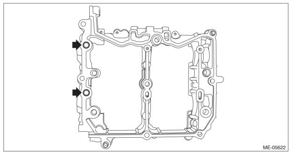
4) Remove the liquid gasket from cam carrier RH and front camshaft cap RH, intake rear camshaft cap RH and exhaust rear camshaft cap RH.
