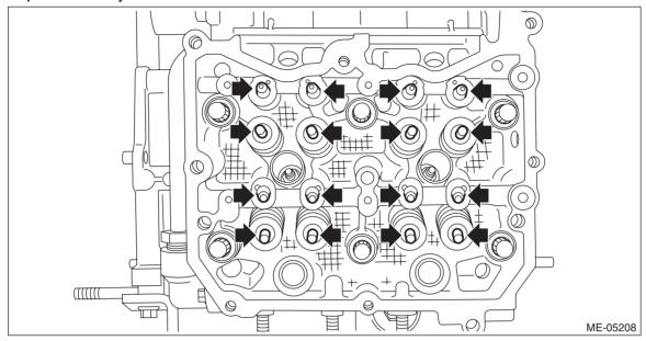
3) Apply engine oil to the O-ring and the roller rocker arm, and install the O-ring and the roller rocker arm to the cylinder head RH.
