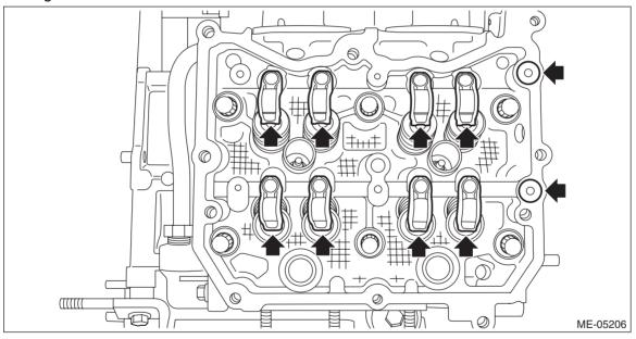
4) Apply liquid gasket to the mating surface of cam carrier RH as shown in the figure.
