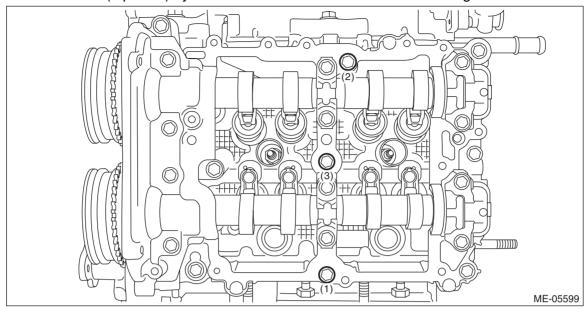
(3) Tighten the bolts (3 places) with a torque of 18  $N \cdot m$  (1.8 kgf-m, 13.3 ft-lb) in numerical order as shown in the figure.
