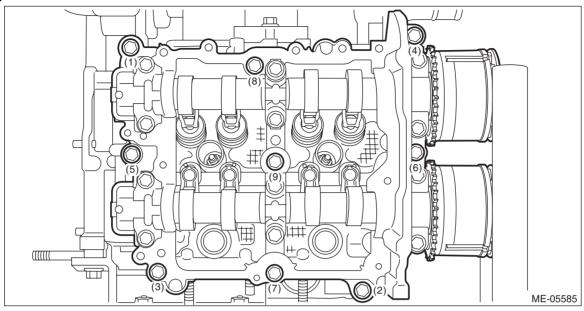
12) Remove the O-ring and the roller rocker arm from cylinder head RH.
