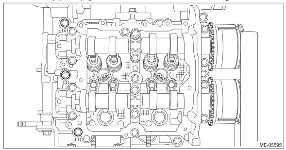
(7) Tighten the bolts (3 places) with a torque of  $18 \text{ N} \cdot \text{m}$  (1.8 kgf-m, 13.3 ft-lb) in numerical order as shown in the figure.
