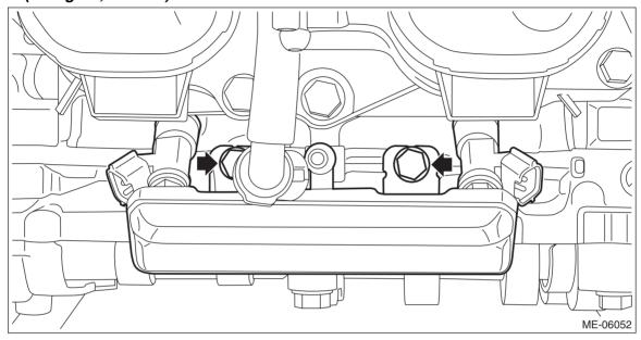
(2) Connect the quick connector to the fuel pipe LH.
