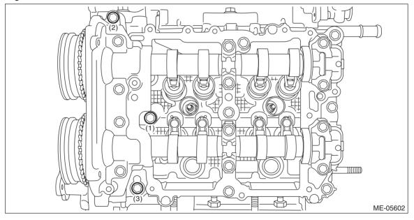
(6) Loosen the bolts (3 places) by 180° in numerical order as shown in the figure.
