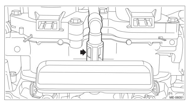
(3) Connect the connectors to the fuel injector LH.
