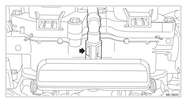
(3) Remove the bolts securing the fuel pipe LH, and remove the fuel pipe LH and the fuel injector LH.
