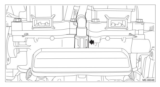
(3) Remove the bolts securing the fuel pipe RH, and remove the fuel pipe RH and the fuel injector RH.
