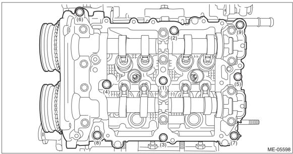
(2) Loosen the bolts (3 places) by 180° in numerical order as shown in the figure.
